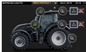
It's easy to configure the work lights using the 9" touchscreen. There are also on/off buttons for the work lights and beacon in the armrest.
